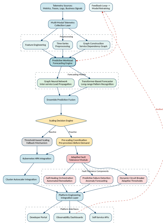
Fig. 1. High-level architecture diagram of the AI-Driven Predictive Autoscaling and Fault Tolerance Framework, showing the five components and their interactions.
